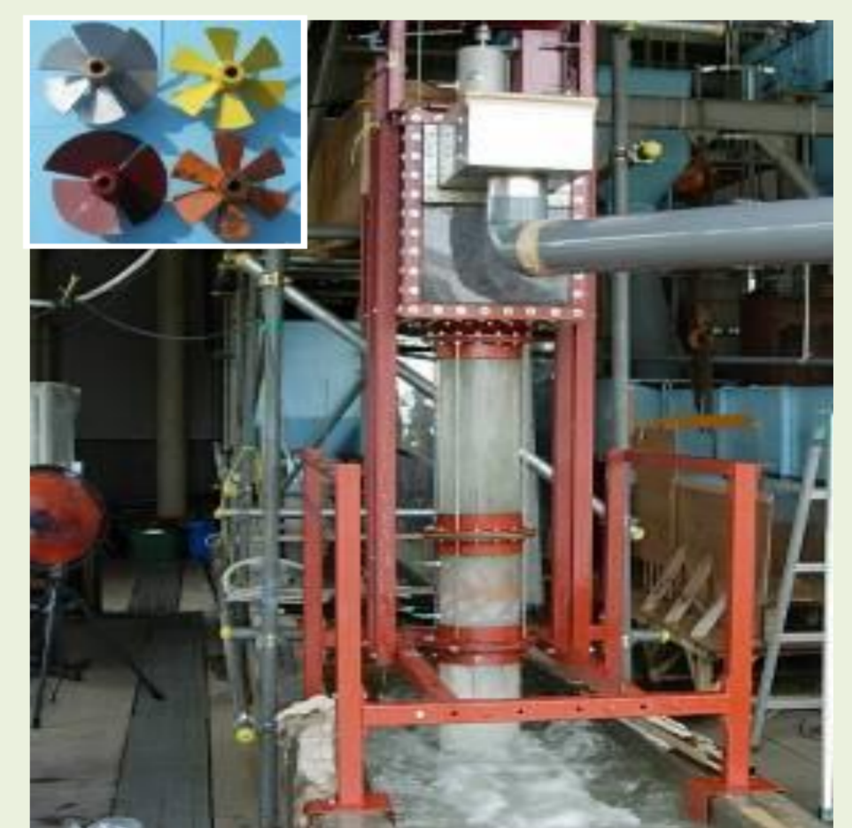
Hydro generation of 1 kW
